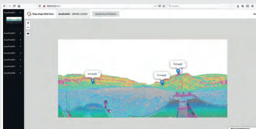
Screenshot from RIEGL SlopeAngle App web-browser. Critical slope-angles over 70° are highlighted; markers can be set interactively to monitor these points over a time-series of scans
