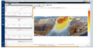
Without leaving the software, users have direct access to its entire suite of safety-critical analysis, charting and alarming tools via the SSR-Viewer tab.
