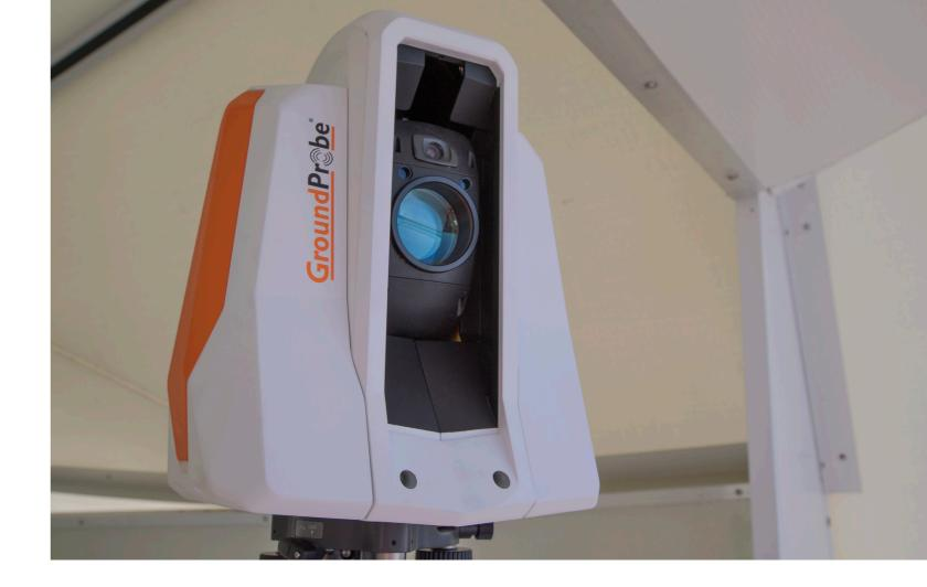
The GMS-Dual monitored continuously and without interruption, successfully detecting sub-millimetre movement, reflecting its high accuracy and precision.
