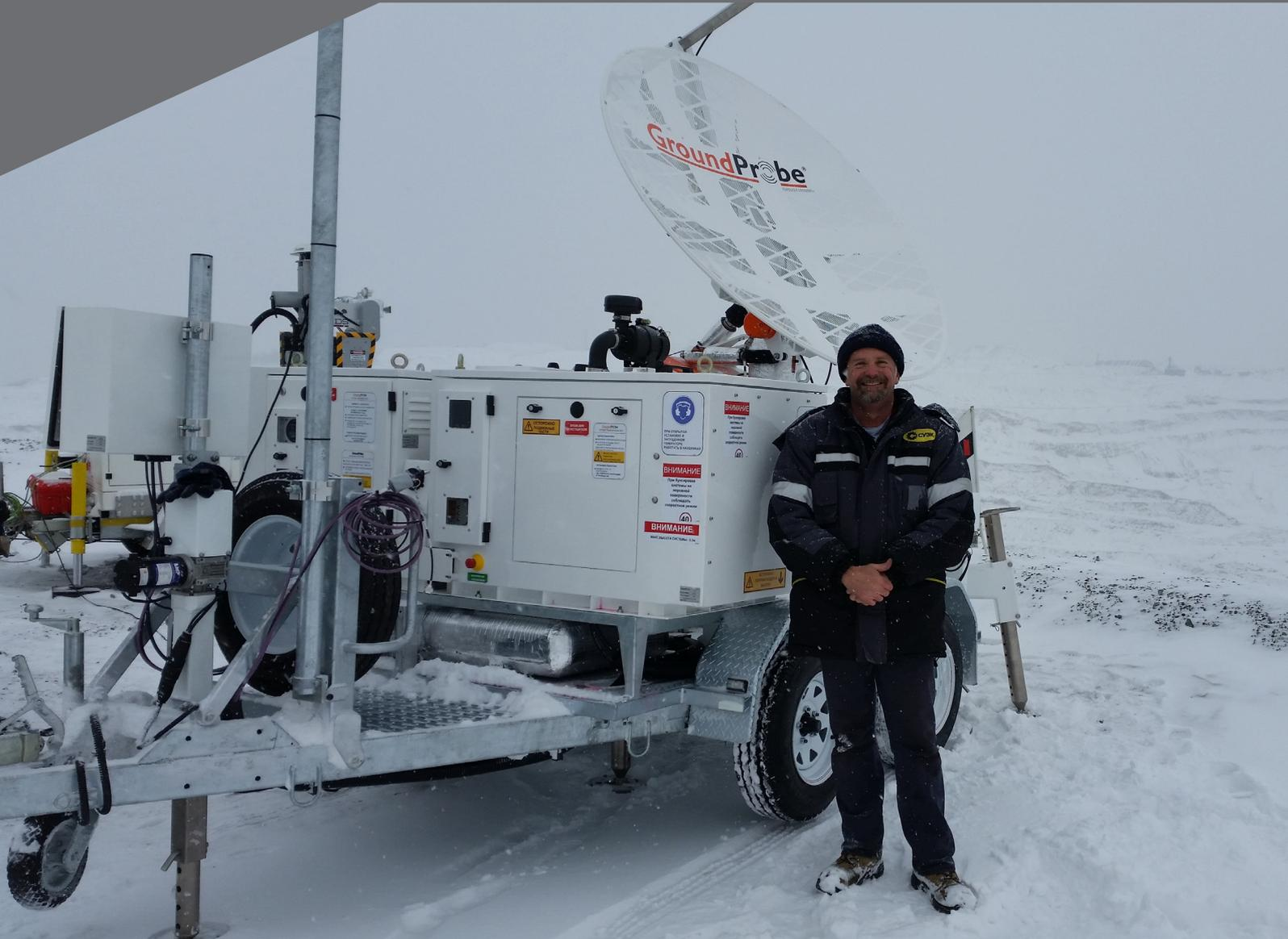
GroundProbe achieved the objective of running all the radar heaters from the CPS with acceptable charge cycles during the coldest months of winter in Siberia, consequently allowing all of the on-site GroundProbe radar systems to run smoothly.
