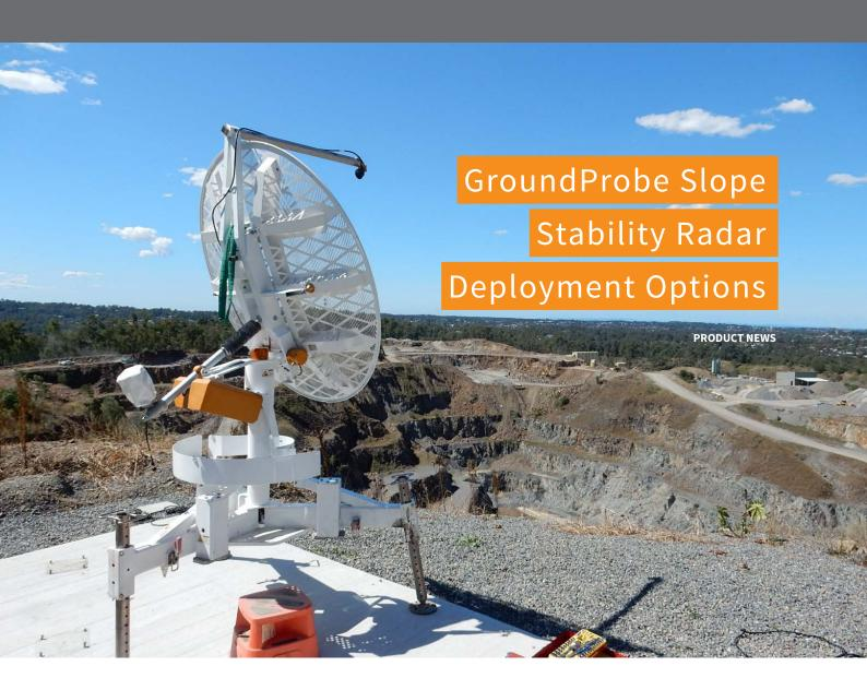
GroundProbe offers two deployment options across our Targeted Monitoring (SSR-XT) and our Broad-Range Monitoring (SSR-FX) radar models; fixed and mobile.
