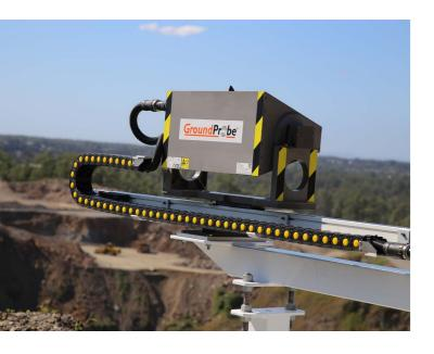
SSR-SARx is available as a fixed installation, where it can be securely mounted in a specific location at a large stand-off distance, effectively monitoring entire dam walls quickly and easily with sub-millimetre precision.
