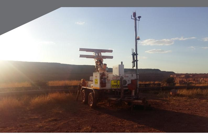
"The SSR-FX is designed to detect unknown hazards and deformation hotspots across vast areas making it extremely useful for early detection of movement or slope failures in large mines like Kolomela," said Clifford Walsh, GroundProbe's Business Manager for Africa and Europe.
