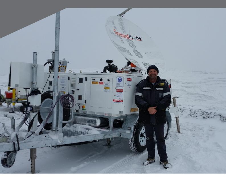
GroundProbe achieved the objective of running all the radar heaters from the CPS with acceptable charge cycles during the coldest months of winter in Siberia, consequently allowing all of the on-site GroundProbe radar systems to run smoothly.
