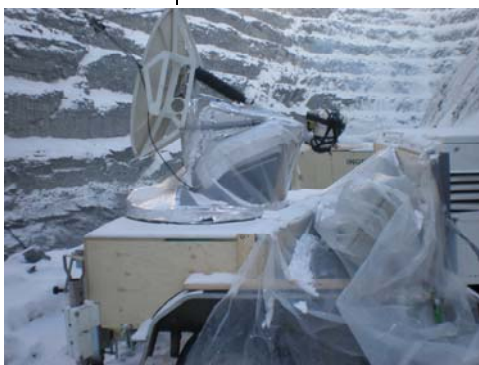
▲ Slope Stability Radar monitoring at Troilus pit
