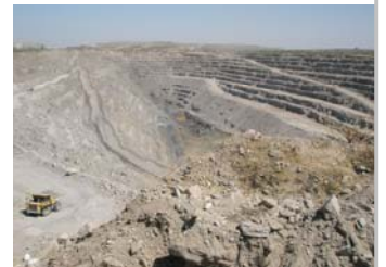
View of RAM pit from the south. The SSR-X system is located on the footwall (east) to monitor the hanging wall (west wall).
